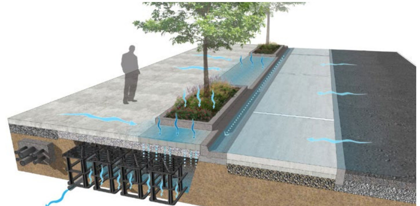
Silva Cell Sytem - Stormwater interception, evapotranspiration, and infiltration Credit: DeepRoot
